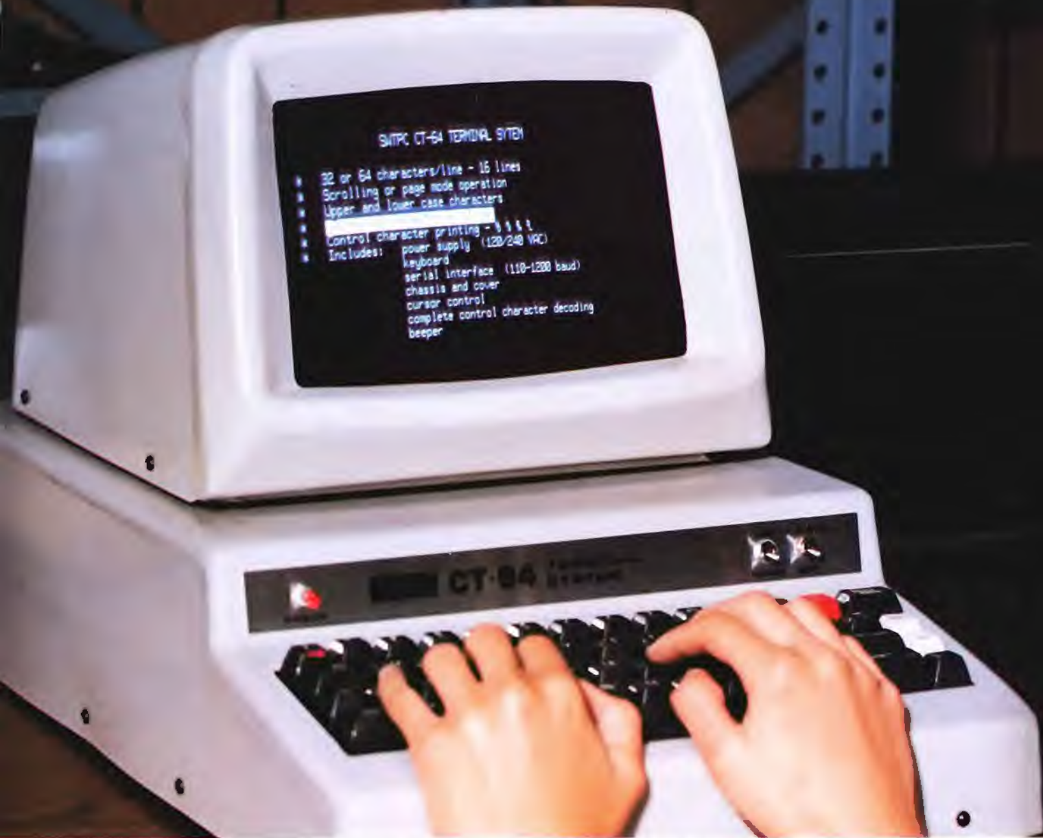
The 9-inch screen of the CT-VM monitor ($175) shown here with Southwest's new CT-64 illustrates the terminal's 64-character lines, switchable control character printing, and word highlighting. At just $500 for both, these matching units provide a complete CRT terminal with full cursor control, 110-1200 Baud serial interface, and many other features.
